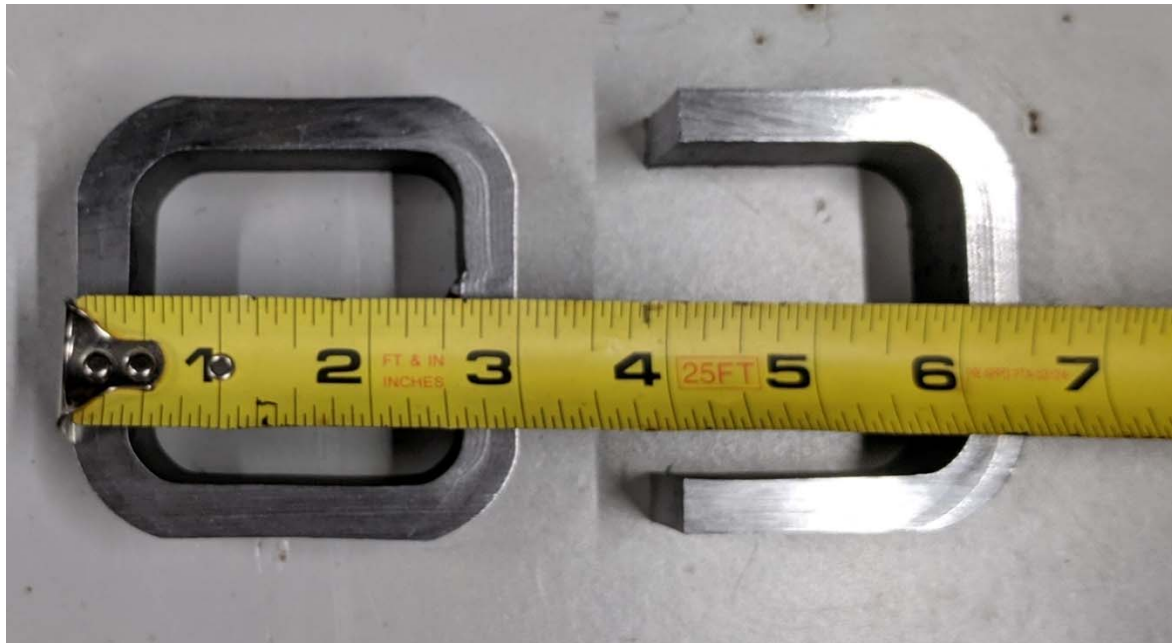
Figure 14: Creating "C" Guides for the Moving Top Platen
