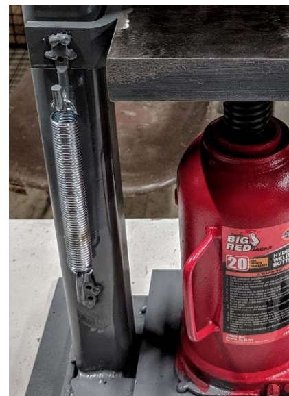
Figure 19: C-277 welded - only slight tension at rest
