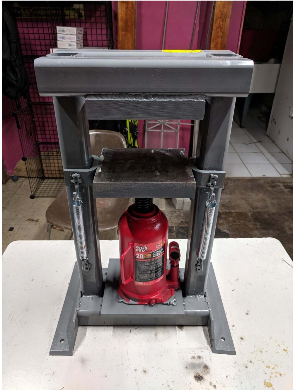
Figure 1: This 20-Ton Hydraulic Press Design with Paint and Springs
